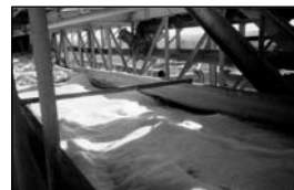
Photo E: TIVAR® 88-2 launderer running full. To date, no signs of wear or corrosion are visible.
