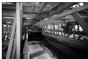
Photo B: The combination of abrasion and corrosion caused by deterioration of the 400 BHN steel used for the launderer
